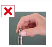
② Use special tools to remove/replace the cutting edge. Use spanners (JIS B4630) for removing/exchanging the cutting edges. For spanner's width size, refer to the H size (shown in back page). Tightening torque: Take special care, otherwise excessive tightening may cause breakage on cutting edge.
